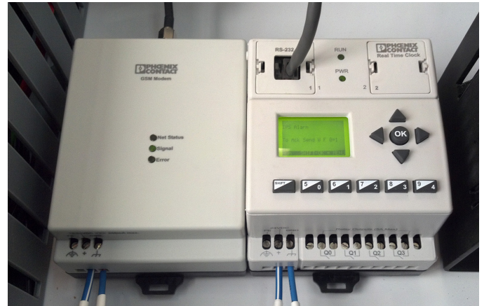
The GSM modem is one of several expansion modules available to make the Nanoline even more flexible.
