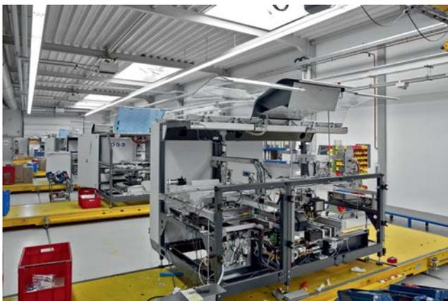
**Figure 3:** A new soldering system leaves the production line in Wertheim, Germany, after nine cycles, each lasting four hours.
