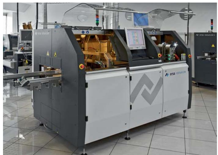
**Figure 2:** Versa-Flow selective-soldering systems
